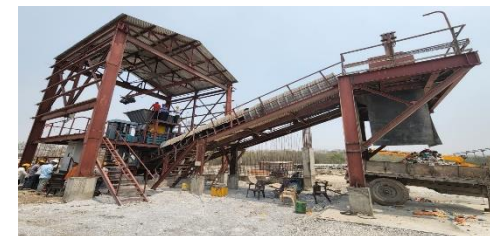
Shredder for co-processing of AFR
